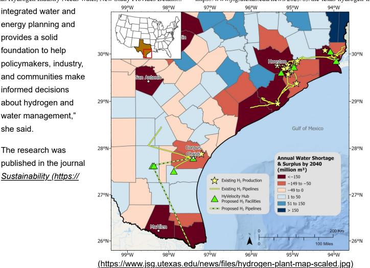
Existing and proposed hydrogen infrastructure as of 2024 in the Gulf Coast region of Texas overlaying projected water needs by 2040 per county. Credit: Lin et al.
